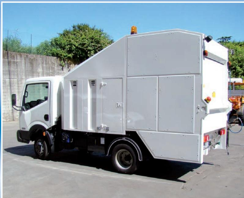
The **Mini35** washing machine has been designed with few and simple targets in mind: B driving licence equipment, cost and weight savings, only available in a configuration with a 2500mm wheel-base, machine width 1800mm.
