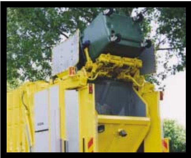
**Mecam 2.** That a horizontal split body offers another advantage. Using an optional separation plate in the tailgate, two Mecam 2 bins (two chamber bins divided parallel to the comb) can be emptied independently. Increasing speed and efficiency even more.
