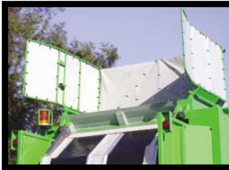
**Details that keep waste where it belongs.** Windscreens on top of the GCP automatically unfold and prevent that waste is blown away during loading. The single piece tailgate opens in two stages - no cross contamination occurs during discharge of the loaded fractions.
